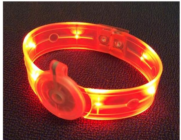
Fig. 8. the WrapLight demonstrator manufactured by R2R hybrid in mould integration.
