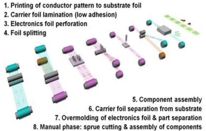
Fig. 2. R2R hybrid integration manufacturing process.
