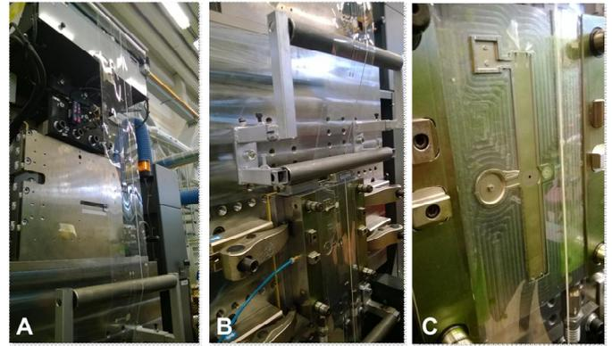
Fig. 6. Picture of the a) R2R foil feeder, b) foil moving to right position and c) fixed cavity side after ejection.
