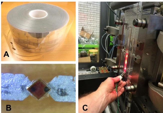
Fig. 7. a) Printed electronics foil b) a microscope image of a LED bonded to the conductor on a foil, and c) testing assembled electronics before overmoulding.
