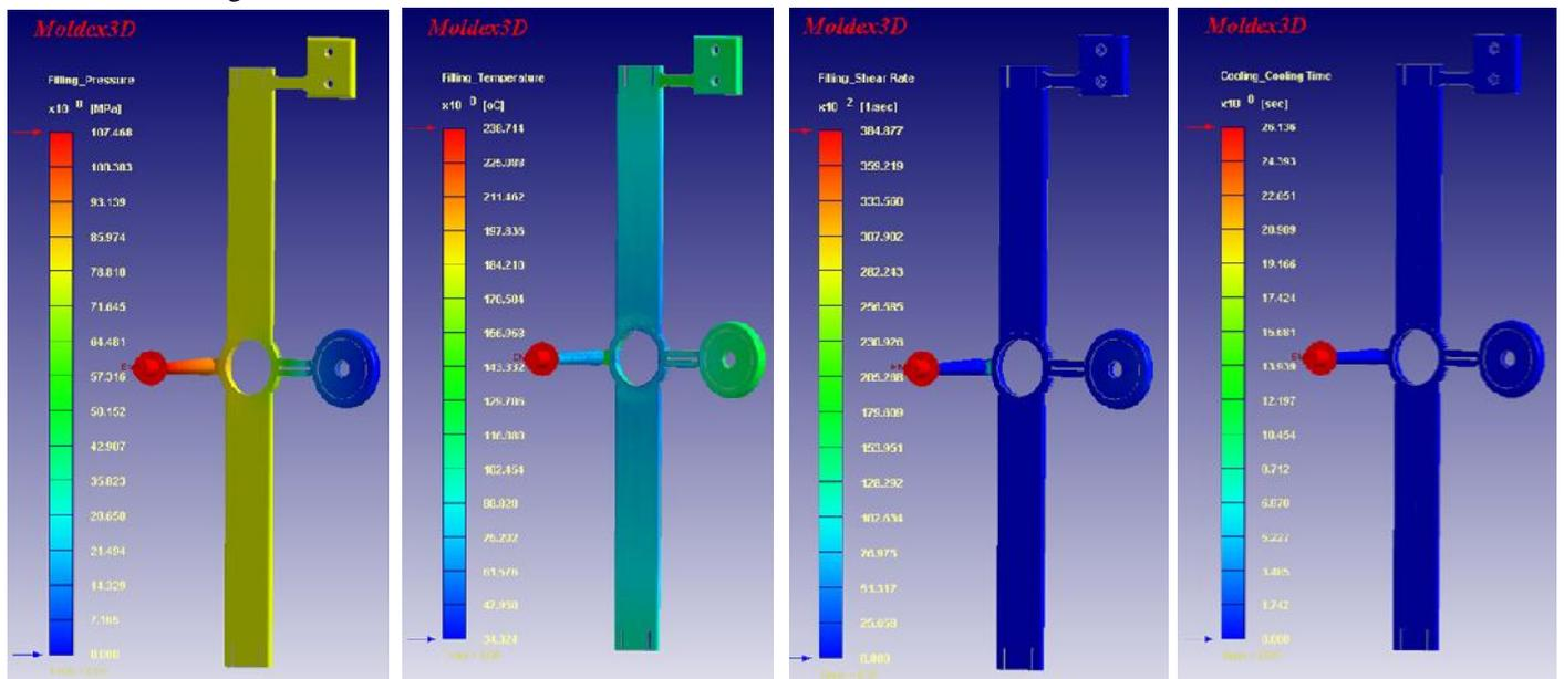
Fig. 5 Results of the mould cavity Moldex3D simulations.
