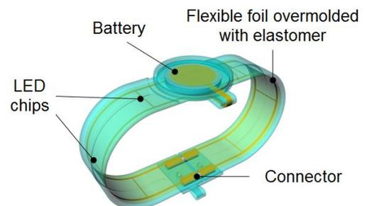
Fig. 3. WrapLight technology demonstrator concept.
